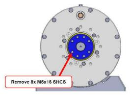
11. Re-assemble the plunger retainer and Drive Rod using 8/off M5x16 SHCS Black. Use Loctite 7471 activator and Loctite 243 thread locker on each fastener Open the inlet valve: **DO NOT DROP ANYTHING (SCREWS OR FOD) IN THE ACTUATOR!** Torque each M5 screw to 9.5Nm or 7ft•lbs and paint mark, and insert BS154 O-ring to the End Cap Insert using FML-2.
