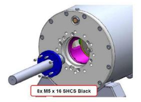
6. Assemble the clamps with 3/off M6x12 SHCS Black. Use Loctite 7471 and 243. Torque each M6 to 16Nm. Paint mark SHCS after tightening.
