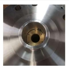
10. Use pliers to hold hardware (screw and lock washer) and place a small amount of Loctite on end of screw. Places screws into internal holes and install them down with Allen key.
