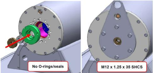
9. Remove the End Cap Insert, Seal Housing, and Guide Bush. Use proper Wrench to remove the Seal Housing.
