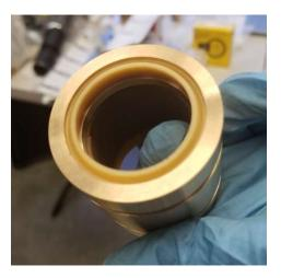
7. Coat O-Rings in versa lube and install on adapter piece insert. Then you may install Adapter Piece Insert into Adapter plate with gas compression seal facing upward
