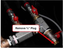
5. Run hose to container full of oil. The oil pump will be used to help fill actuator with oil.
