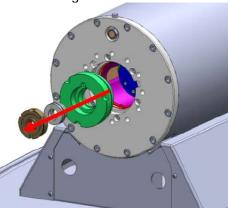
4. Remove the plunger retainer plate by removing the 8/off M5x16 SHCS fasteners.
