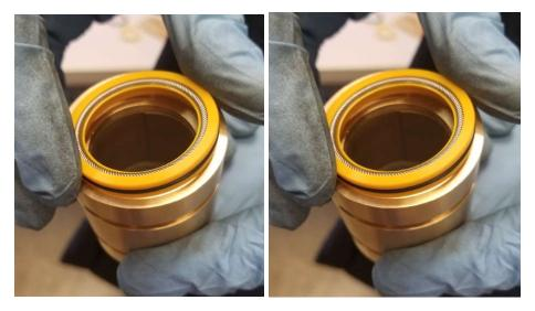
5. Turn over the Adapter Piece Insert and find the edge with a lip. Install the Wiper Seal with the steps facing outward.
