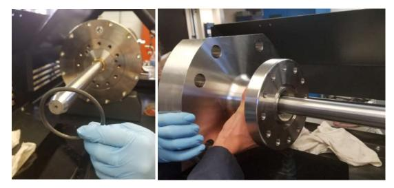
12. Insert O-ring into adapter plate, press until approximately 2 inches are left between the dive and adapter plate.
