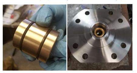
8. Use hammer and tool to install the Adapter Piece Insert so it is flush with internal surface (shown below).
