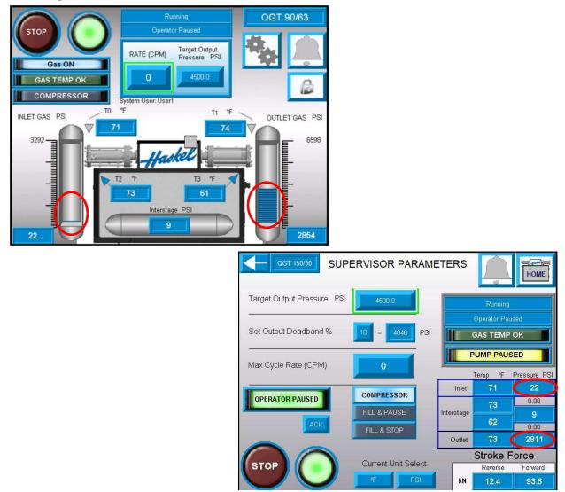
Comparison of Home Screen and Supervisor Parameters Screen for Gas Pressure
