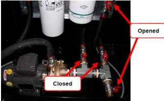
7. Loosen the Breather Plug and start hand pumping the oil. Keep observing the sight through glasses which you can view the oil level on Actuator.
