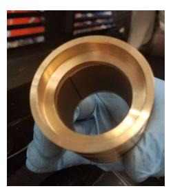
4. On edge with NO LIP, install gas compression seal with the spring facing outward. It should be flush upon final installation.
