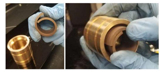
3. Install ring until edges are flush and ring is flat against internal diameter.
