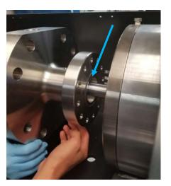
13. Obtain 12 bolts and lock washer and assemble as above. Place anti-seize on the end of the bolt. Install all screws into adapter plate and hand tighten.
