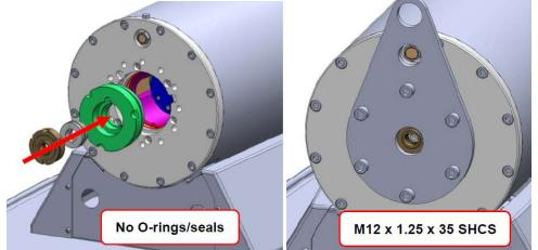
3. Remove the End Cap Insert, Seal Housing, and Guide Bush. Use proper Wrench to remove the Seal Housing.
