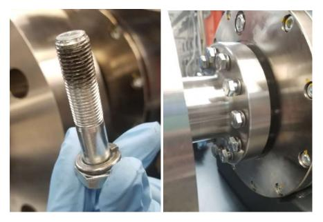
14. Insert screw from under panel so that end is visible on top side of panel. Turn screw into bolt until it is supporting adapter piece as shown below.
