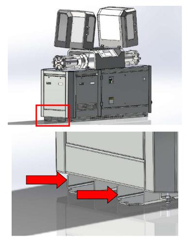
2. Also at the bottom on the front of the unit, the unit can be lifted from.
