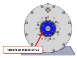
5. Re-assemble the plunger retainer and Drive Rod using 8/off M5x16 SHCS Black. Use Loctite 7471 activator and Loctite 243 thread locker on each fastener Open the inlet valve: DO NOT DROP ANYTHING (SCREWS OR FOD) IN THE ACTUATOR! Torque each M5 screw to 9.5Nm or 7ft•lbs and paint mark, and insert BS154 O-ring to the End Cap Insert using FML-2.
