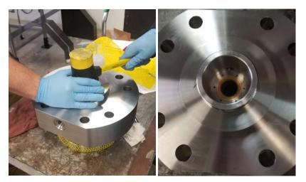
9. Install Adapter Insert Cap. Align holes with adapter plate below.
