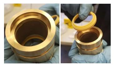
6. Wiper seal should sit flush with edge as shown below.
