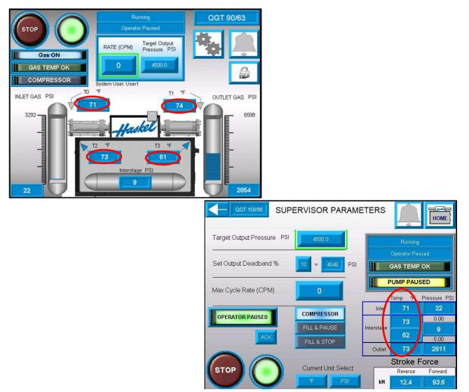
Comparison of Home Screen and Supervisor Parameters Screen for Gas Temperature
