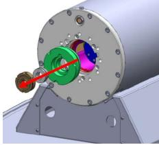
10. Remove the plunger retainer plate by removing the 8/off M5x16 SHCS fasteners.
